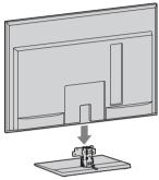
3 Fix the TV to the Table-Top Stand according to the arrow marks ★ that guide the screw holes using the supplied screws.
